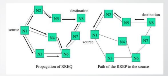
Figure 1: AODV Routing Protocol
